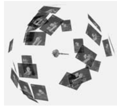
From left to right - 3D optical measurement with blue light fringe pattern projector and stereoscopic cameras - turbine seen from the scanner cameras - dome of images acquired by the sensors - Example of mesh repair on the turbine rotor - Comparison between the scanned turbine mesh and the repaired CAD
